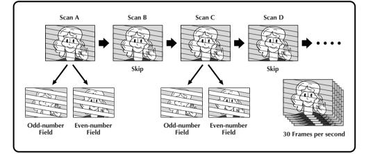
Scan A is recorded, divided into an odd- and even-number Field, and then Scan B is skipped. Scans C and D are handled in the same way as Scans A and B, as illustrated above, thereby recording 30 Frames per second.
